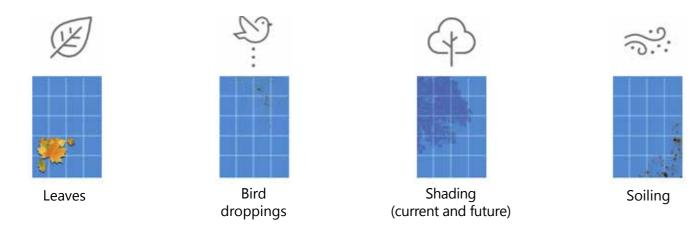
With traditional inverters, the weakest panel reduces the performance of all panels. With SolarEdge, each panel produces the maximum energy, and power losses are eliminated.
